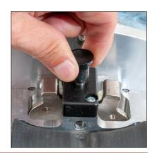
The strand locks aren't used in the over-lashing procedure and must remain in the open position.
