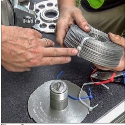
1. If the lashing wire is wrapped with wire ties, rotate the head of the wire tie attached to the looped end of the lashing wire to the center of the coil (see figure 3). This will facilitate the cutting of the wire tie in a later step and help ensure that the complete wire tie is removed.
