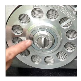
1. Once the lashing wire is loaded onto the Super G lasher, it is time to route the wire through the machine for proper operation. Pull enough wire off the reel to make the termination of the wire to the strand. Pass the wire under the tension adjustment roller then over the guide roller.
